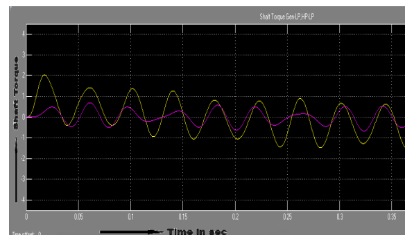
Figure 5. Shaft torque of system without fault
