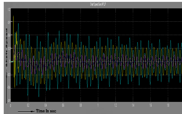
Figure 14. Shaft speed of system with three phase to ground fault
