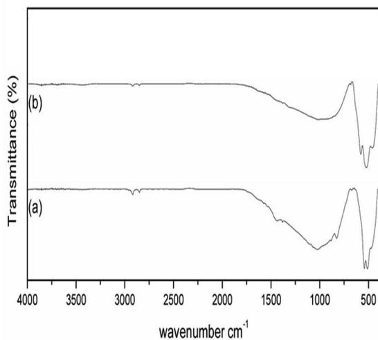
Figure 3: FTIR spectra of (a) pure Bi<sub>2</sub>O<sub>3</sub>, (b) 5.0 wt% In-doped Bi<sub>2</sub>O<sub>3</sub> calcinated at 600 °C.
