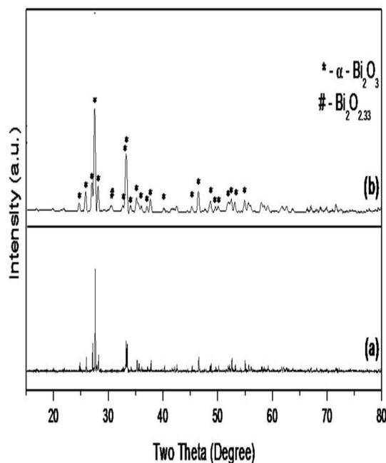
Figure 1: XRD patterns of (a) pure Bi<sub>2</sub>O<sub>3</sub> and (b) 5.0 wt% In-doped Bi<sub>2</sub>O<sub>3</sub> calcinated at 600°C.
