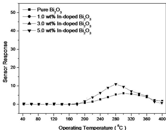
Figure 5: Sensor response of In-doped Bi<sub>2</sub>O<sub>3</sub> to 50 ppm C<sub>2</sub>H<sub>5</sub>OH as a function of operating temperature.
