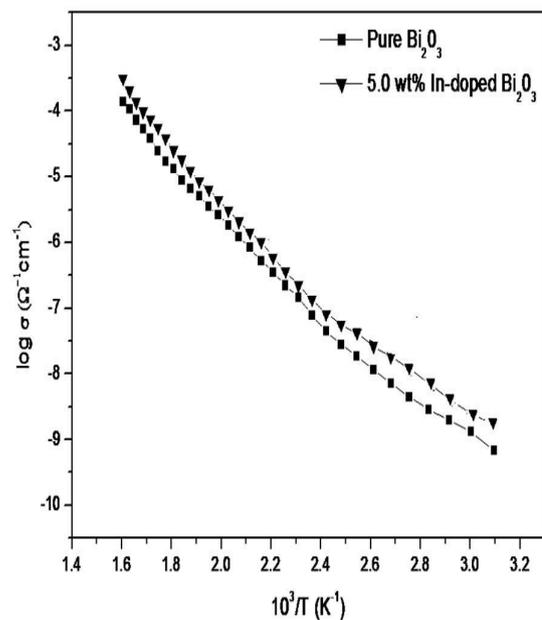
Figure 4: Variation of log (σ) versus 10<sup>3</sup>/T for pure and In-doped bismuth oxide thick films.
