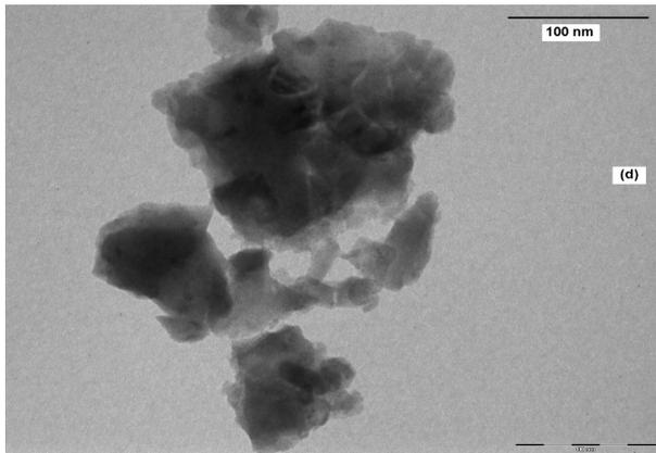
Figure 2: TEM images of 5.0 wt% In-doped Bi<sub>2</sub>O<sub>3</sub> calcinated at 600 °C
