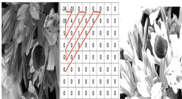
Figure 3: DCT working procedure (Input image, zigzag order scanning, Re-construction image of input image by using 1/4 DCT coefficients)
