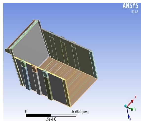
Figure 1: Pro-E Model of A36 Tipper Body
