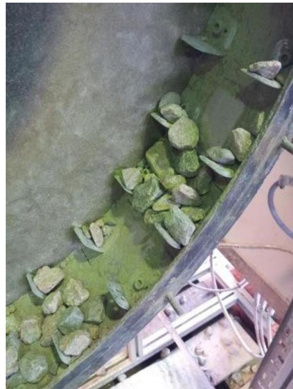
Figure 4: Lifters Hindering the Sliding of Abrasive Particles
