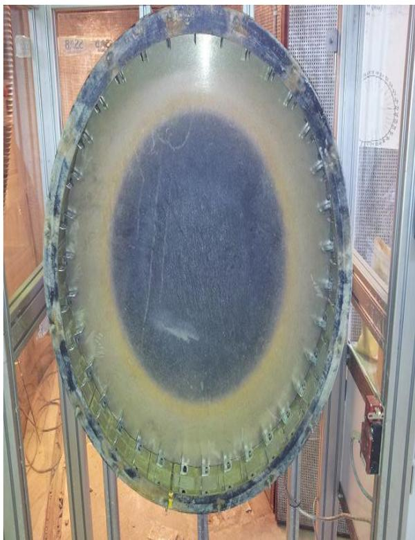
Figure 3: The Drum with a Total 68 Lifters Assembled
