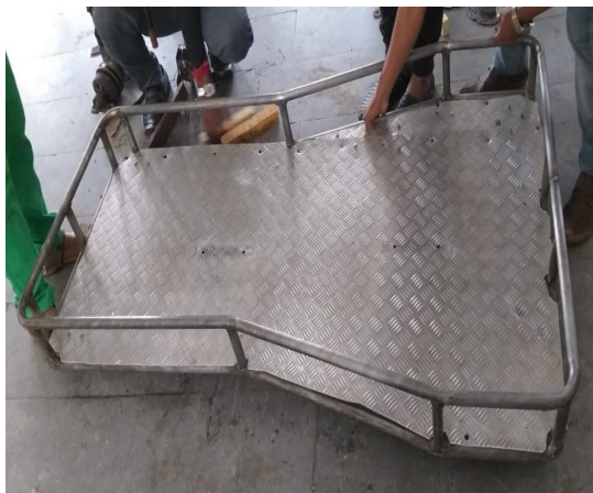
Figure 12: Chassis with Sheet for Cockpit
