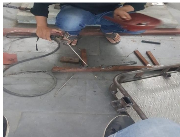
Figure 9: Chassis Rod Welding
