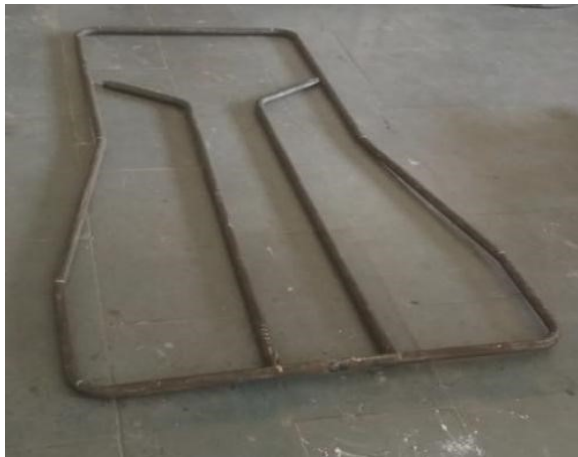
Figure 10: Pipes Bend for In-process Chassis
