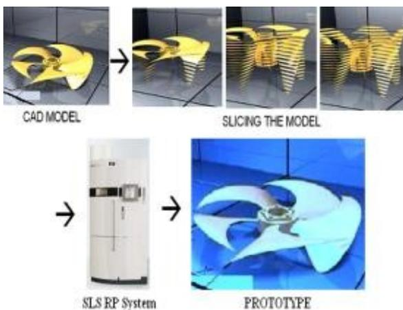
Figure 2: Selective Laser Sintering Modelling Process
