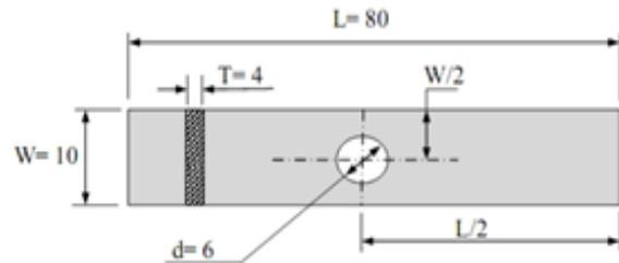
Figure 3: Test sample drawing for dimensional Analysis (all dimensions are in mm)
