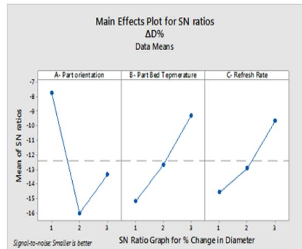
Figure 6: S/N Ratio for graph for % change in diameter
