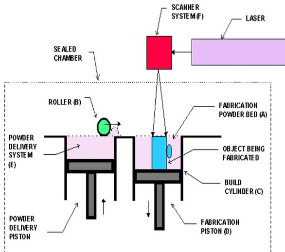
Figure 1: Selective Laser Sintering
