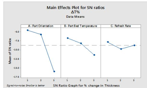
Figure 8: S/N Ratio for graph for % change in Thickness
