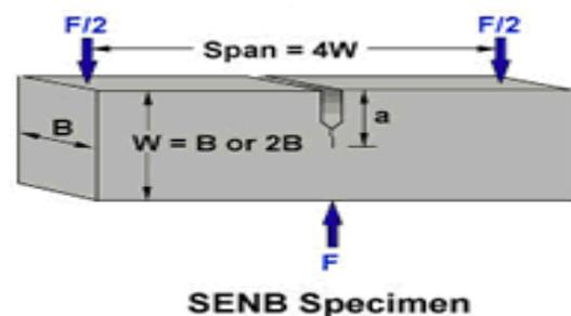
Figure 1: Three-point bend test specimen configuration
