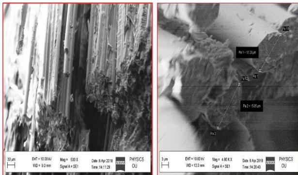
Figure 3: SEM micrographs of Mode-I fracture surface for composite ( $0^\circ$  orientation fibers)
