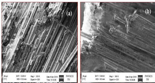
Figure 4: SEM micrographs of Mode-I fracture surface for composite (a)  $45^\circ$  and  $90^\circ$  orientation of fibers
