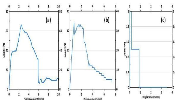
Figure 2: Load Vs. Displacement(mm) curve of composites having (a) 0° (b) 45° and (c) 90° orientation of fibers
